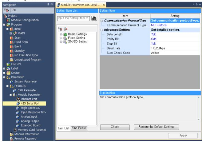
Step 3. [Online] > Transmit the parameter set to [Write to PLC] and reset the PLC.
