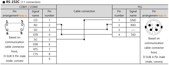
\*Note 1) The pin arrangement is as seen from the connecting side of the cable connection connector.
