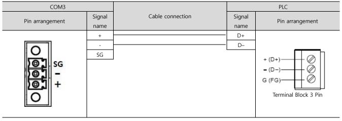
**RS-485** 1 : N connection - Refer to 1:1 connection to connect in the following method.
