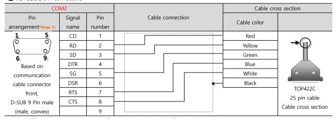
\*Note 1) The pin arrangement is as seen from the connecting side of the cable connection connector.
