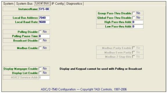
**Step Reference.** The communication settings are set in 'System/Local Baud Rate', and other data bits, stop bits, and parity bits are fixed values.
